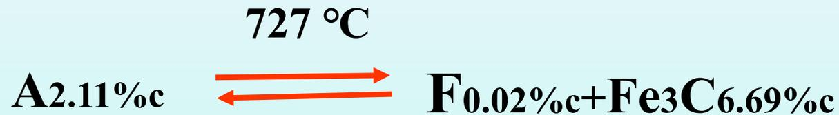
共析反应的产物即珠光体  $\text{P} = \text{F}_{0.02\%c} + \text{Fe}_3\text{C}_{6.69\%c}$
